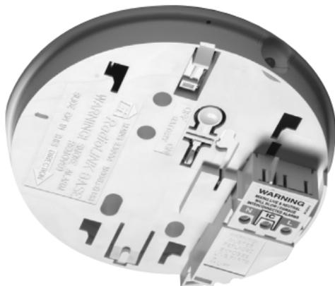
The primary function of the RadioLINK base is to interconnect all Alarms in the system, i.e. when one Alarm senses fire, the EIB168RC base attached to that Alarm will transmit an RF signal that will activate the sounders in all the other Alarms.
