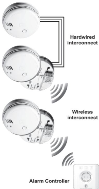
In this configuration the alarm controller must be a RadioLINK device.
