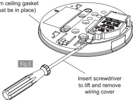
The wiring must be TPS 1.5mm<sup>2</sup> and connected to the terminal block on the mounting plate as follows:
