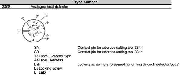
Prepared for mechanical locking, when plugged in the analogue base 3312. One hexagon socket locking screw is attached (1.5 mm Hex key to be used). One 2.5-2.7 mm hole has to be drilled.
