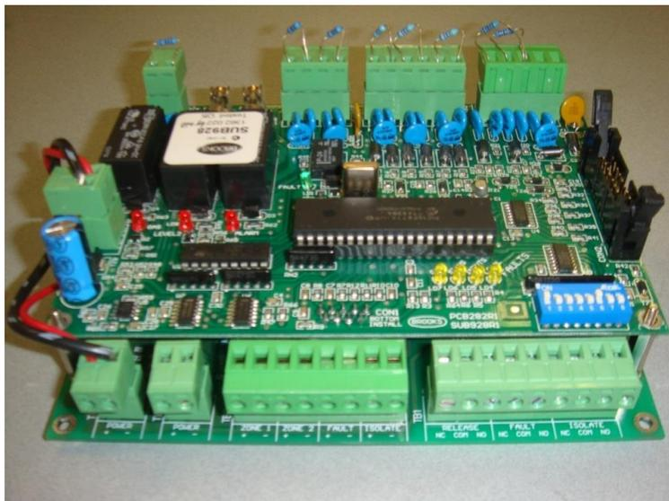
Figure 29 Assembled Control & Interface Boards
