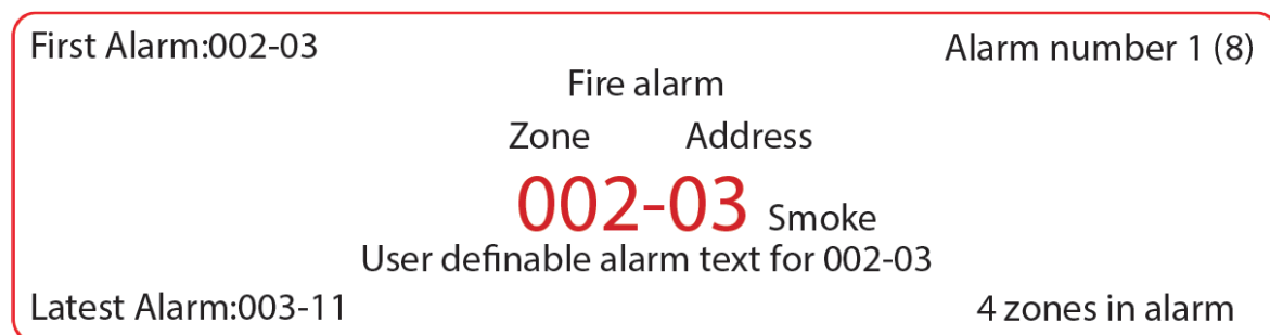
Figure 11: More than One Alarm Point Activating Fire Alarm.
