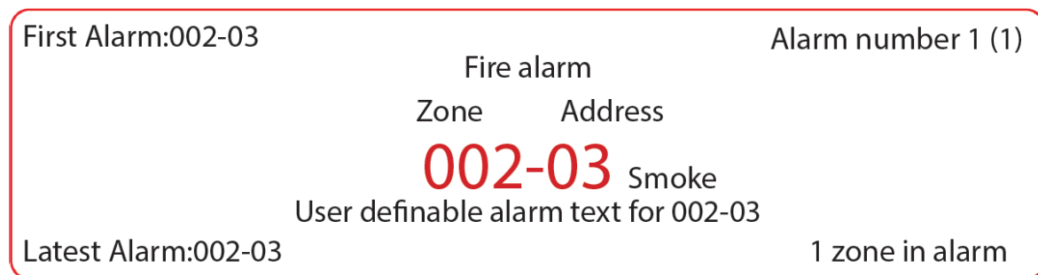
Figure 10: One Alarm Point Activating Fire Alarm (fire alarm zone 002, address 03).
