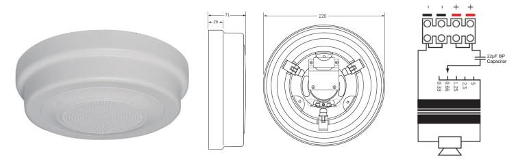
Designed to meet the requirements of AS ISO7240.24:2015 the SPKSM100QF features a flame retardant housing material and a tuned PA driver to suit the new approval requirements. One-Shot design simply snap-fits in seconds to the surface mounting ring, reducing installation time considerably.
