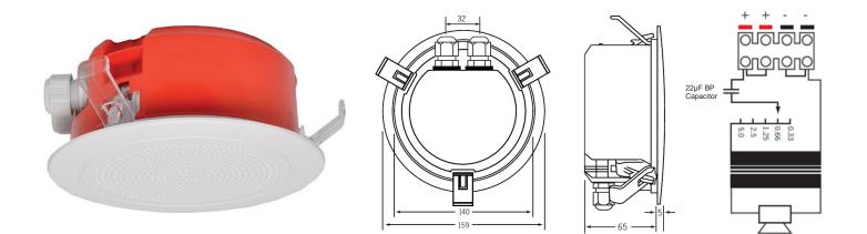
The SPKFM100QF low profile flush mount ceiling speaker is certified to AS ISO7240.24:2015. Each speaker is fitted with a fire retardant speaker/transformer dome and oversized cable glands and terminal blocks for easy on site termination. One-Shot design allows the speaker to simply snap-fit into the ceiling once the terminating is completed.
