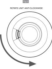
IF THE UNIT HAS BEEN TAMPERPROOFED, IT WILL NOT TWIST OFF - SEE FIGURE 8c
