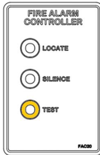
Figure 10 Wiring fault of the external trigger
