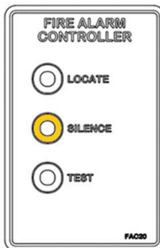
Figure 11 Firmware fault of FAC20
