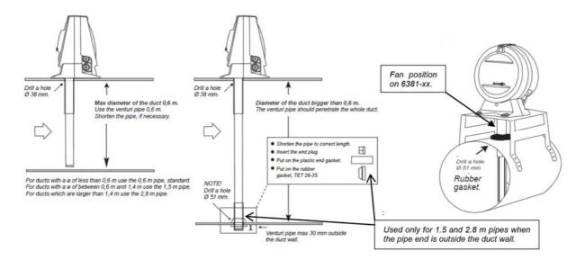
Left: How to suit the pipe to different widths of the ventilation duct. 6377 can be mounted vertical on the duct and 3 x the duct diameter before or 5 x the duct diameter after a disturbance, i.e. a fan, a bend, a filter, a silencer, a damper, etc.
