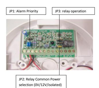
The input/output module is a zone device which interfaces BARFS-1 to external equipment. The module is fitted (clip in) in x-series rectangular plastic base.
