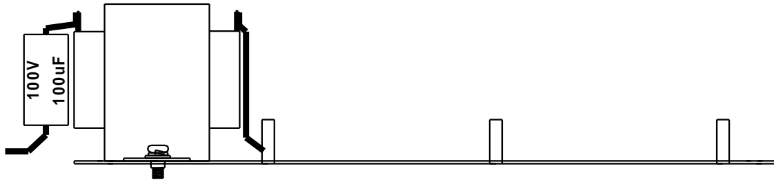
Figure 14 60W Transformer Fitted into Brooks Equipment Plate
