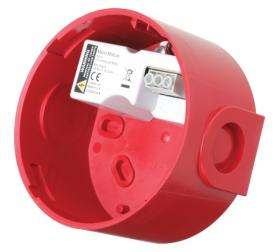
The Mains Deep Base incorporates a small 24Vdc supply that allows any of the compatible sounders and strobes to be operated from 110 or 230Vac supplies. This allows the installer much greater flexibility in the use of products and their applications.
