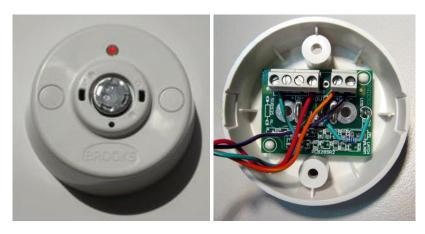
The residential heat detectors will be mounted and pre wired to RFP6 interface card. Only two wires are internally connected to SUB332, positive and interconnect.
