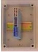
**2822 Isolated Zone Interface.** The Isolated Zone Interface (2822) contains a waterproof box (IP66/67) that is supplied with four compression glands for the cable entries, an Isolated Zone Interface board (2823) mounted on a DIN rail, a DIN rail interface intended for an I/O unit 3361 and one 8K2 EOL resistor. The box has to be mounted outside the hazardous (Ex) area
