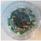
A control expression for activation has to be programmed, similar to a programmable output or alarm device. It takes one COM loop address. For more technical data, see the Product Datasheet.
