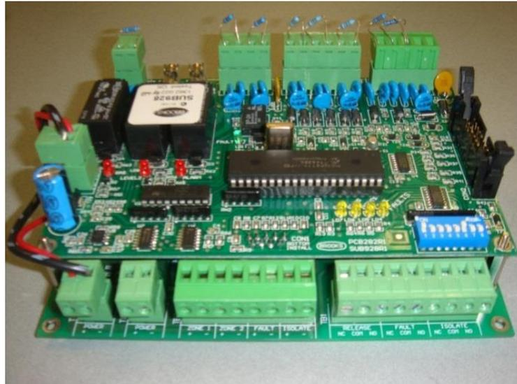
Figure 22 Assembled Control & Interface Boards
