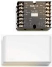
Addressable 2 voltage outputs unit. The unit is connected directly to the COM loop. External 24 V<sub>DC</sub> supply is required (via a 3366AU unit or FT128).
