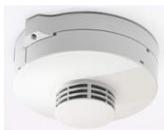
**4352** Photoelectric smoke detector. **Discontinued** and replaced with 4452. Scattered light (i.e. reflection of infrared light) is used to detect smoke. An advanced alarm algorithm is used to secure the smoke detection and to reduce false alarms, e.g. a minimum of nine consecutive readings over the fire alarm level are required before the detector goes into alarm. (One reading per sec.). To be plugged in a conventional detector base 2324.
