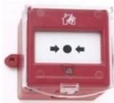
**4439** Enclosed Addressable Manual Call Point with isolator<sup>45</sup>. Replaces 3339. 4439 is same as 3339 unit but it has built-in Short Circuit Isolator. The isolator does **not** use any COM loop address. The Address setting tool 3314 / 4414 is also used for mode setting same as 4433.
