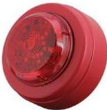
**4380** Addressable beacon<sup>65</sup>. 4380 is a visual alarm device of type A for indoor use. All electronics, the LEDs and the lens are mounted in a red ABS housing. The beacon comes with a shallow base (IP21C). A deep base is an option which gives the beacon a higher IP protection (IP33C). 4380 is powered via the COM loop, i.e. the number of beacons is dependent on the type and number of other units connected to the COM loop but 10 maximum.
