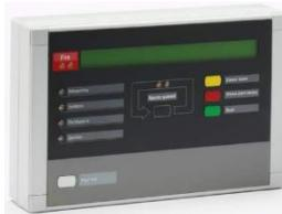
**1736** Alert Annunciation Unit (AAU). A compact size enclosure 145H x 220W x 50D mm made of grey high impact ABS. Fitted with a supplementary "O" ring gasket, it complies with IP61, in respect of dust and moisture. The unit has no door, i.e. the front is accessed directly but the push buttons are disabled until they are supposed to be used. The unit should be wall mounted. Two compression glands are included.
