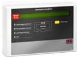
External Presentation unit (EPU). Same enclosure as 1736 except that there are 2 more buttons on the 1736 not exist in 1728, the Silence Alarm Devices and Reset buttons also the Acknowledge button is renamed in 1728 to Silence Buzzer. The push buttons are disabled until an alarm event is received. The unit is to be wall mounted. Two compression glands are included.
