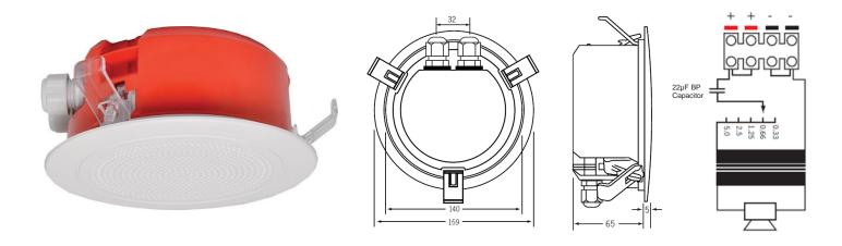
The SPKFM100QF low profile flush mount ceiling speaker is certified to AS ISO7240.24:2015. Each speaker is fitted with a fire retardant speaker/transformer dome and oversized cable glands and terminal blocks for easy on site termination. One-Shot design allows the speaker to simply snap-fit into the ceiling once the terminating is completed.
