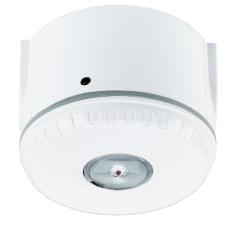
The 4481 Addressable Ceiling Mount Visual Alarm Device (VAD) with isolator has a unique lens design that distributes the light in a cylindrical shape to achieve the required illumination specified by EN54.23. Designed for installation at a height of up to 3m and with a discrete appearance, the device is ideal for a variety of applications, including bedrooms, bathrooms and toilets.
