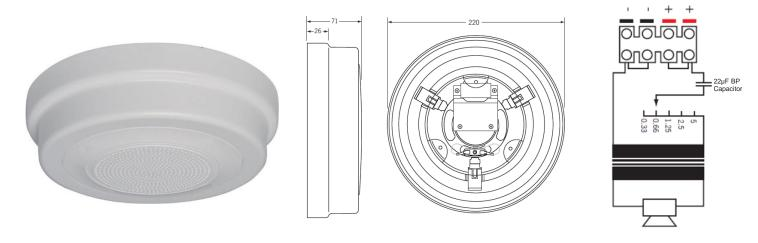
Designed to meet the requirements of AS ISO7240.24:2015 the SPKSM100QF features a flame retardant housing material and a tuned PA driver to suit the new approval requirements. One-Shot design simply snap-fits in seconds to the surface mounting ring, reducing installation time considerably.
