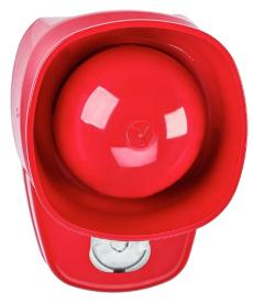
The 4482 Wall Mount Addressable Visual Alarm Device (VAD) with Siren and Isolator has a unique lens design that distributes the light in a cylindrical shape to achieve the required illumination specified by EN54.23. Its durable design and high sound output sounder make it suitable for open areas or where there is higher than normal background noise.
