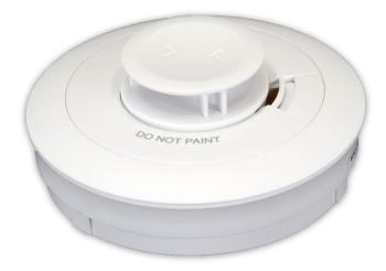
The EIB603CX is an externally powered fixed temperature heat alarm, designed to be used with the Brooks range of Residential Fire Panels, when used in conjunction with a compatible interface base. Fixed temperature heat alarms are designed to trigger when the temperature reaches 58°C. Heat alarms are not sensitive to smoke which make them suitable for kitchens and areas where smoke alarms may be subjected to nuisance alarms. Heat alarms must only be used supplementary to smoke alarms.
