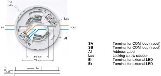
The base is prepared for mechanical locking of the detector, when a detector with a locking screw is plugged into the base. Terminal wire diameter 0.6 - 1.6 mm (approx.  $0.3 - 2 \text{ mm}^2$ ). Analog detectors can be plugged in the base 3312, e.g. 33xx and 44xx.
