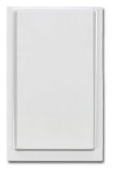
The 4620AU Addressable Base Station interfaces wireless devices to a COM loop in FT1020G3 or FT128. Up to 4 base stations can be monitored on each COM loop and up to 16 Wireless photoelectric smoke detectors on each base station. The base station comes with a built-in short circuit COM loop isolator.
