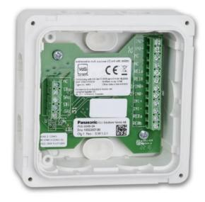
The 4461 loop powered multipurpose input/output module comes fitted with in an IP 65 enclosure. The unit offers two monitored inputs, one isolated voltage input and two programmable relay outputs making it suitable for a range of different applications. The device can be programmed as a fire fan control and status interface module or reconfigured as a 3361 generic input/output module making it backwards compatible with older systems and software versions.
